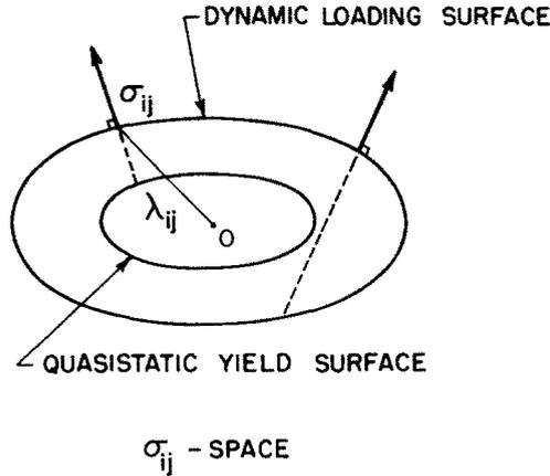
FIG. 1. The quasistatic yield surface and the dynamic loading surface (Perzyna's theory).
