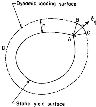
FIG. 6. A static yield surface with corner.
